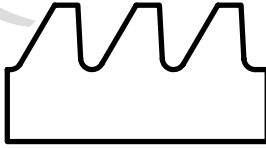
锯齿螺纹 buttress thread
